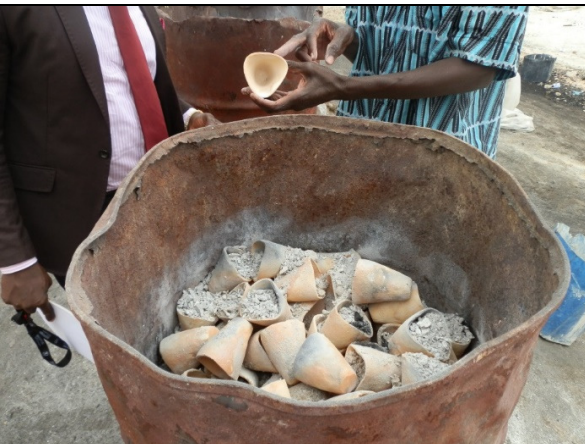
Figure 4: Crucibles after firing in barrel
