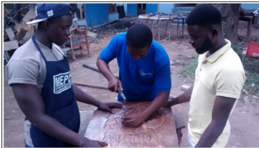
Figure 10: The Chasing and Repoussé of the design
