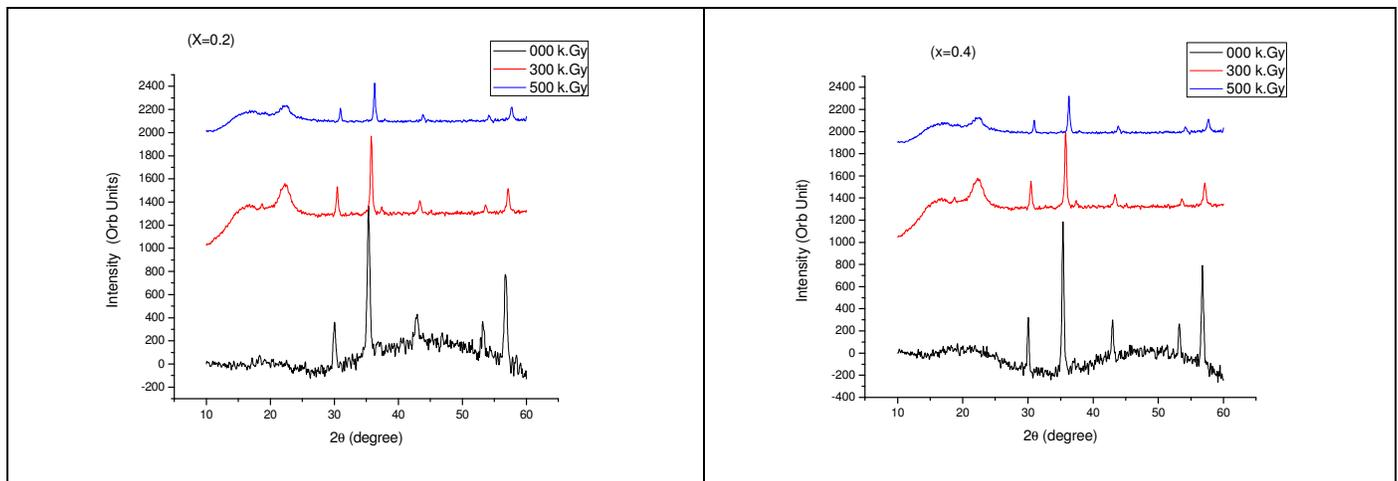
Figure 1: XRD pattern for un- irradiated and irradiated samples of Mg-Zn ferrite
