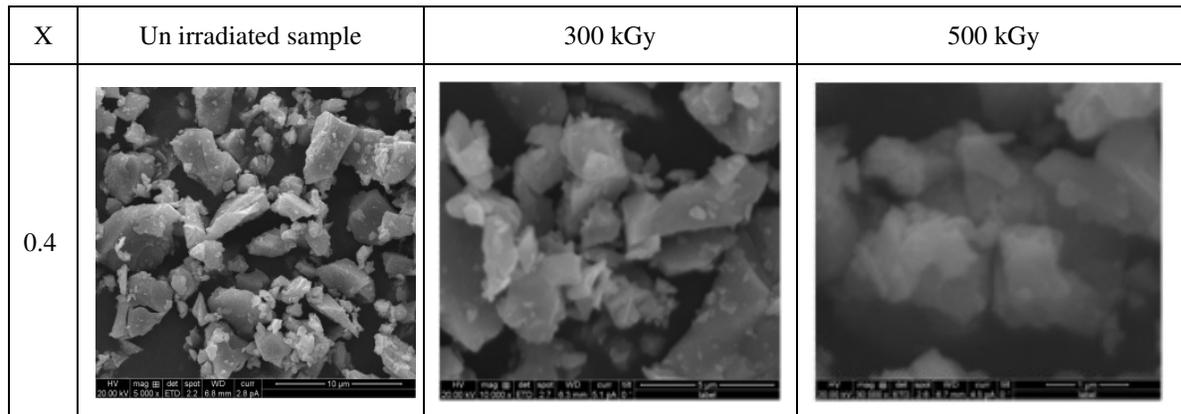
Figure 2: SEM morphology of synthesized ferrite. (Before and after irradiation)
