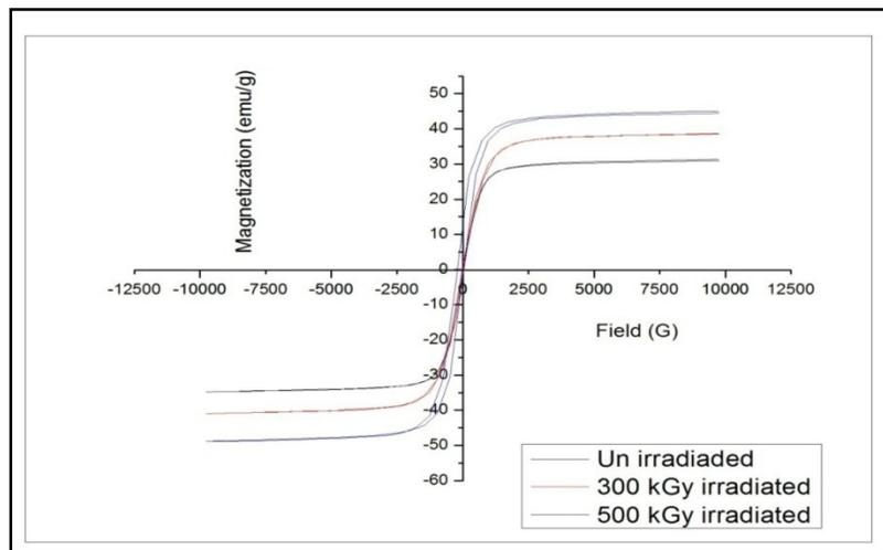
Figure 3: Hysteresis loops for before and after irradiation of  $x=0.6$
