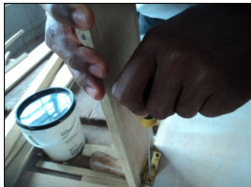
Figure 7: Fixing the hinge on the vertical support and the top part of the stand
