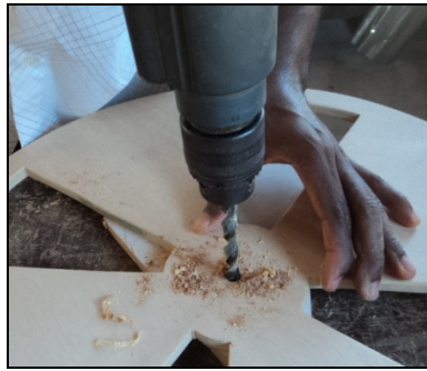
Figure 15: Drilling centre of components of colour wheel
