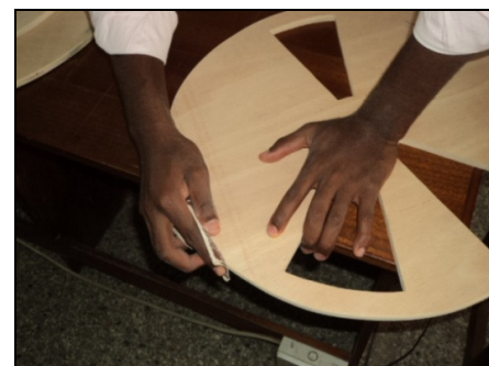
Figure 14: Smoothing surface and edges of components of colour wheel with sandpaper
