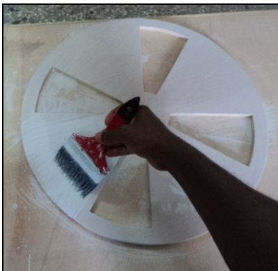
Figure 17: Painting components of colour wheel with emulsion paint
