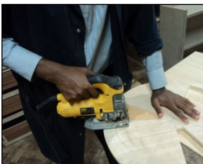
Figure 13: Cutting portions of components of colour wheel with jigsaw
