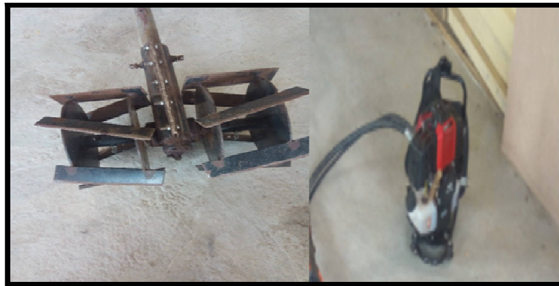
Figure 1: The Weeding Blade, Driving Rotor and 2 Stroke Engines
