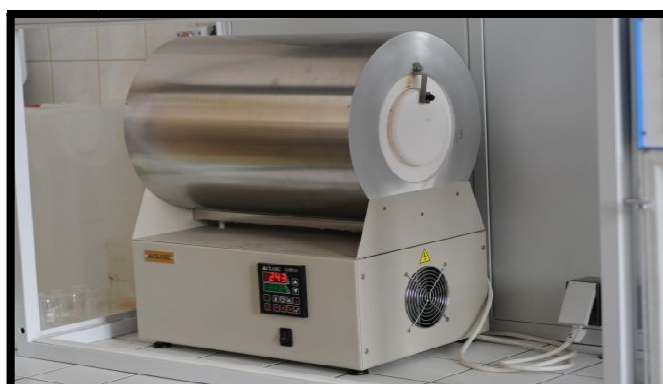
Figure 2: Furnace Used to Calcine TiO 2 Particulate Layers for SEM Analysis (Tum & Oduor, 2014)
