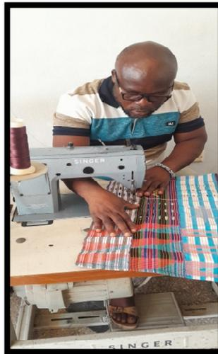
*Figure 21: Joining the Woven Strips*
