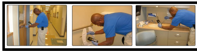
Figure 2: Door Testing, Water Closet Testing, and Wash Hand Basin Testing with an ATP Meter Source: Hygiena, 2022
