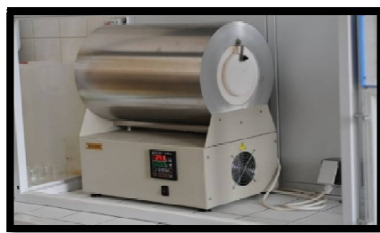
Figure 5: Furnace Used for Annealing TiO_2 Coated Layers
