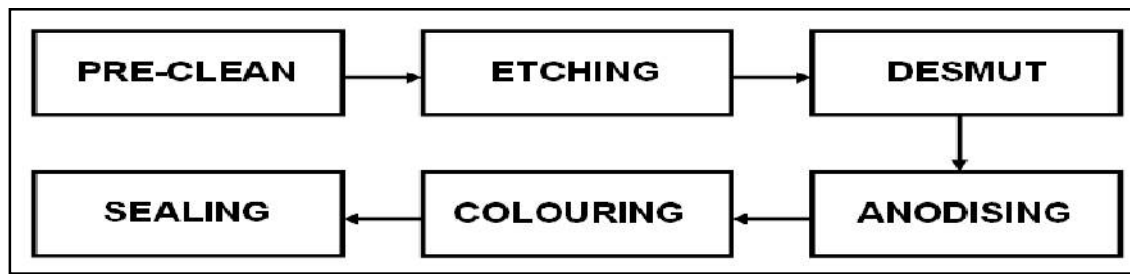
Figure 1: Anodizing process flow diagram (Patel, 2008)
