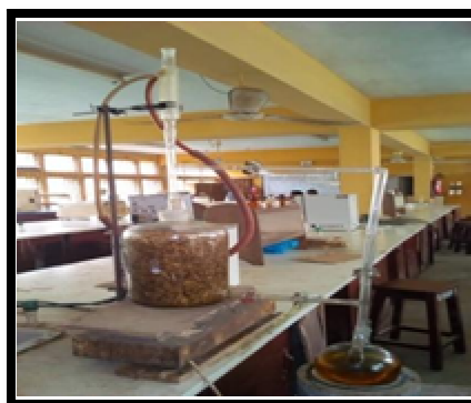
Figure 2: Extraction of the Pulverized Root of Using N-Hexane
